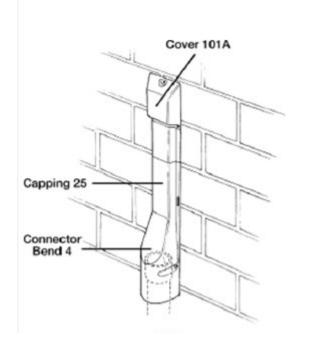
Cable Entry Cover & Capping for running telephone cabling into a premise.
